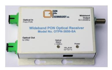
The Olson Technology, Inc. Model OTPN-**3850-**SA provides 50-3,850 MHz bandwidth, allowing it to carry CATV signals from 50-870 MHz along with two stacked 950-2,150MHz L-Band signals. The L-Band signals are usually at a level below the CATV signals.
