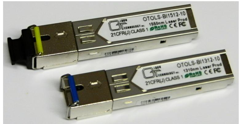
The Olson Model OTOLS-BIYY-ZZD Bidirectional 1.25Gb/s Single-Mode Small Form Pluggable (SFP) Fiber Optic Transceiver is one of several module options available for the Model OTDV-1250 as well as a number of Olson fiber optic Ethernet transport products. The module is compatible with gigabit Ethernet and 1000BASE-SX. The SFP module may be swapped in the field.
