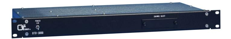
The model **OTD-3000** is a full featured agile demodulator series that is available in four standards, NTSC, PAL B/G, PAL I, and PAL D. The **OTD-3000** will demodulate NTSC frequencies from 55.25MHz (Ch. 2) to 801.25MHz (UHF Ch. 69), and PAL frequencies from 48.25MHz to 855.25MHz, including all cable channels. Sub-Band input and/or Remote Control capabilities are available as optional features. Locally controlled channel selection is by front panel DIP switches.
