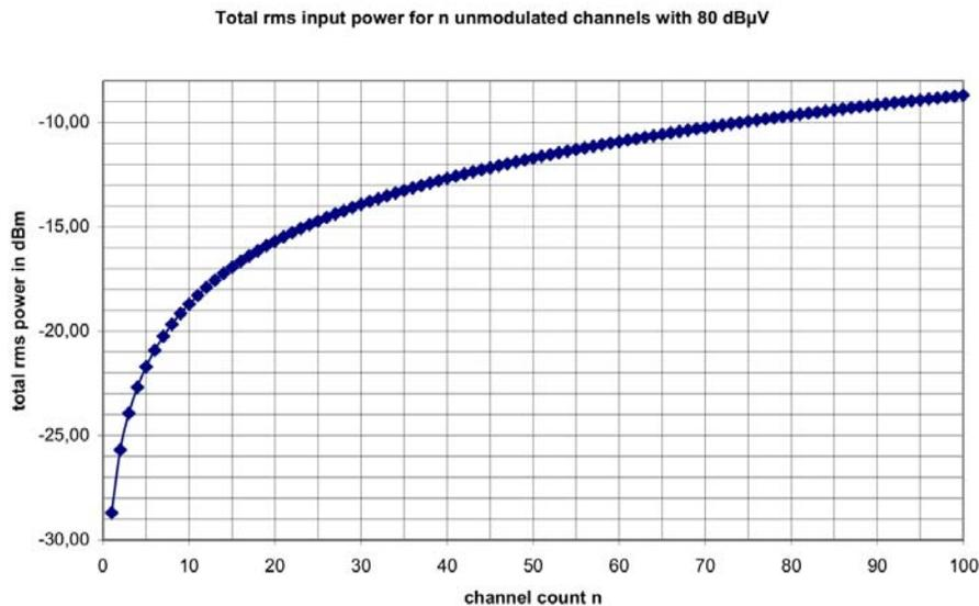
Figure 18 — Total RMS Input Power for N Unmodulated Channels with 80dBμV
